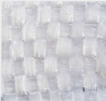
Detalle ampliado del tejido Impregnado Bio Glass Special Discs Enlarged detail of the fabric Bio Glass Special Discs impregnated
